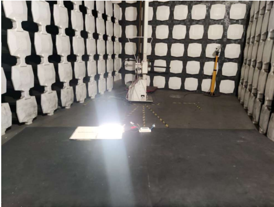
Figure B-3 Setup for Radiated Emission
