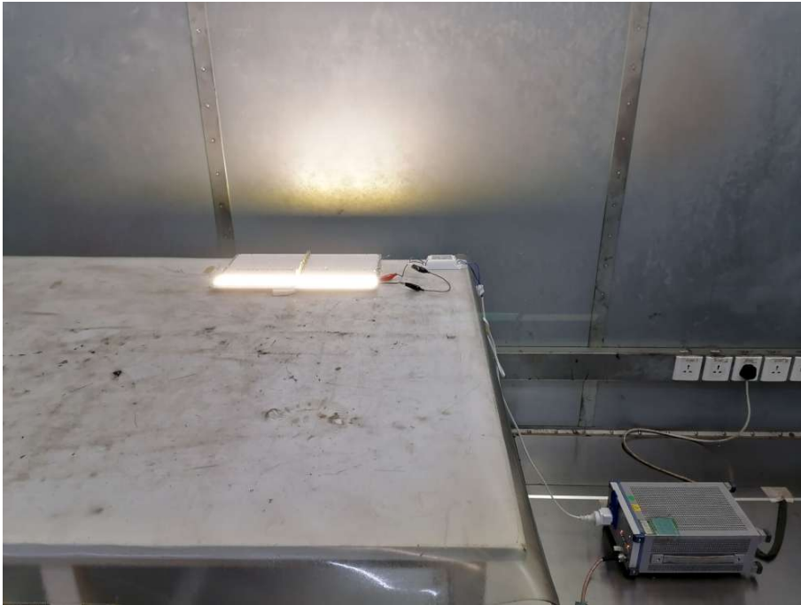
Figure B-1 Setup for Conducted Emission
