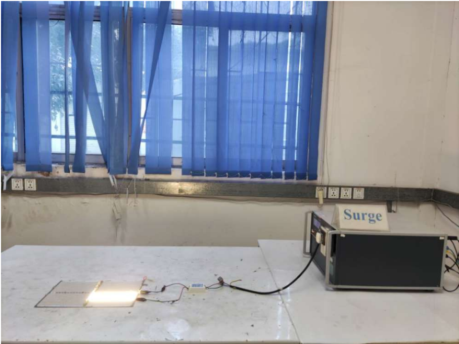
Figure B-8 Setup for Surge
