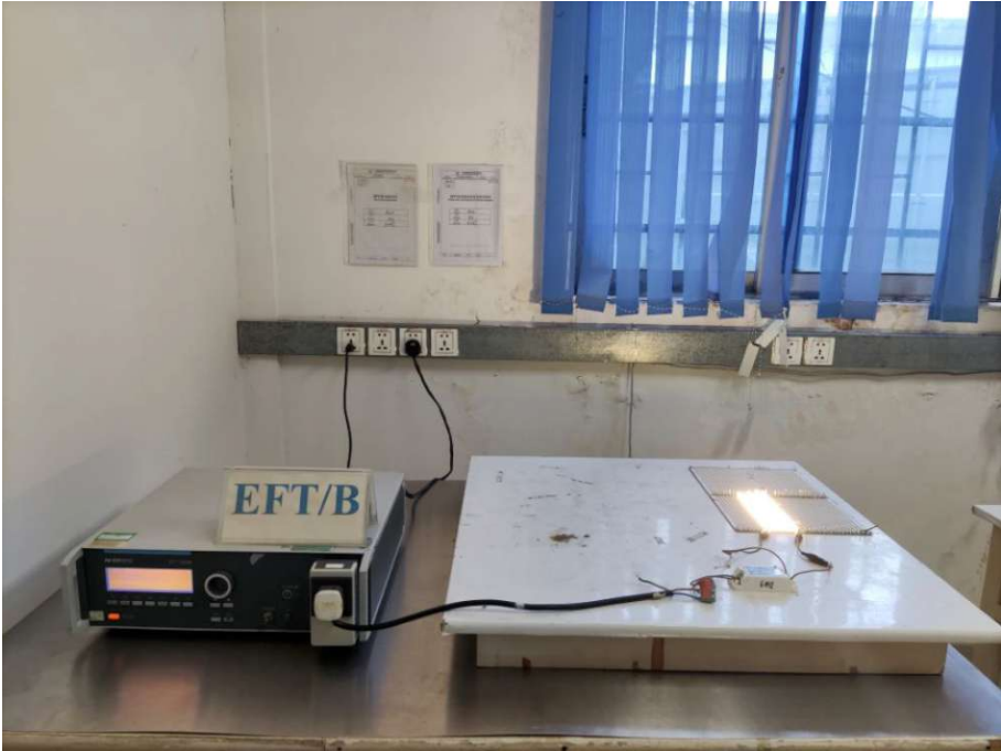
Figure B-7 Setup for Electrical Fast Transients/Bursts
