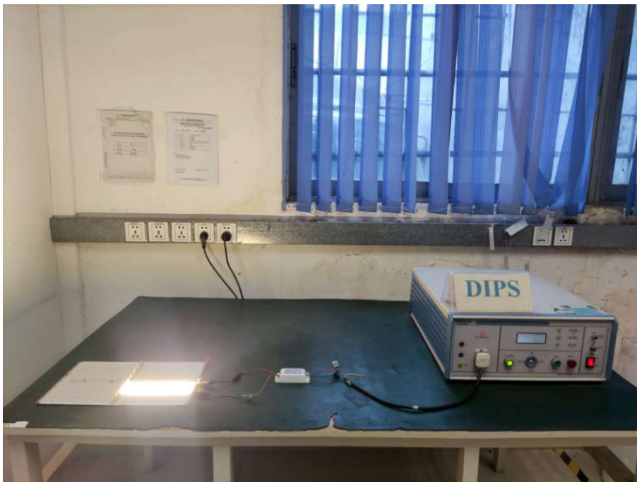
Figure B-9 Setup for Conducted immunity
