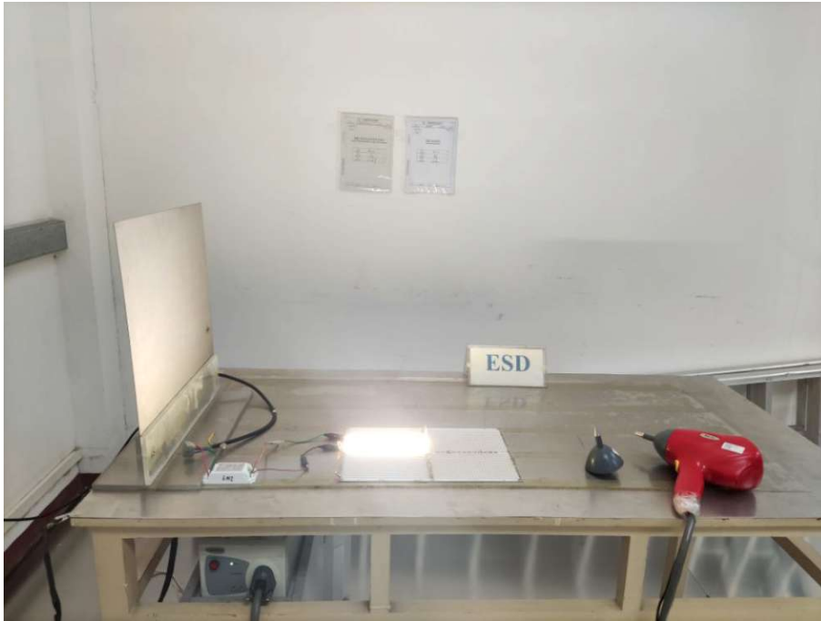
Figure B-5 Setup for Electrostatic Discharge
